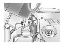
4. Then fill the coolant recovery tank to the COLD FILL line.
